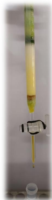
Figure 7. Column chromatography setup for isolating terpene compound L-Carvone by using increasing polarity of the eluent by beginning with pure benzene and ending with ethanol.
