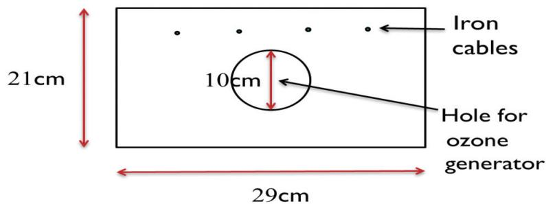
**Fig. 1:** Front view of the cardboard box
